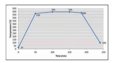
NB: The final heating phase must be adjusted according to the position of the glass in the bending mould.
