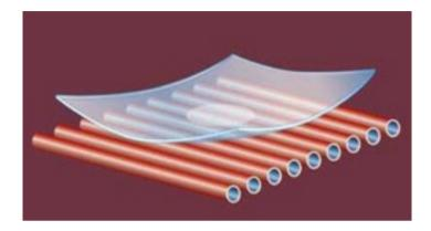
The only way to neutralise these defects is to balance the heating process by using additional heat transfer onto the upper surface. Significantly increasing the temperature of the roof does not resolve the problem because the low-emissivity coating will still reflect this increase in radiated energy. Moreover, this will cause the rollers to overheat which could aggravate the problem.
